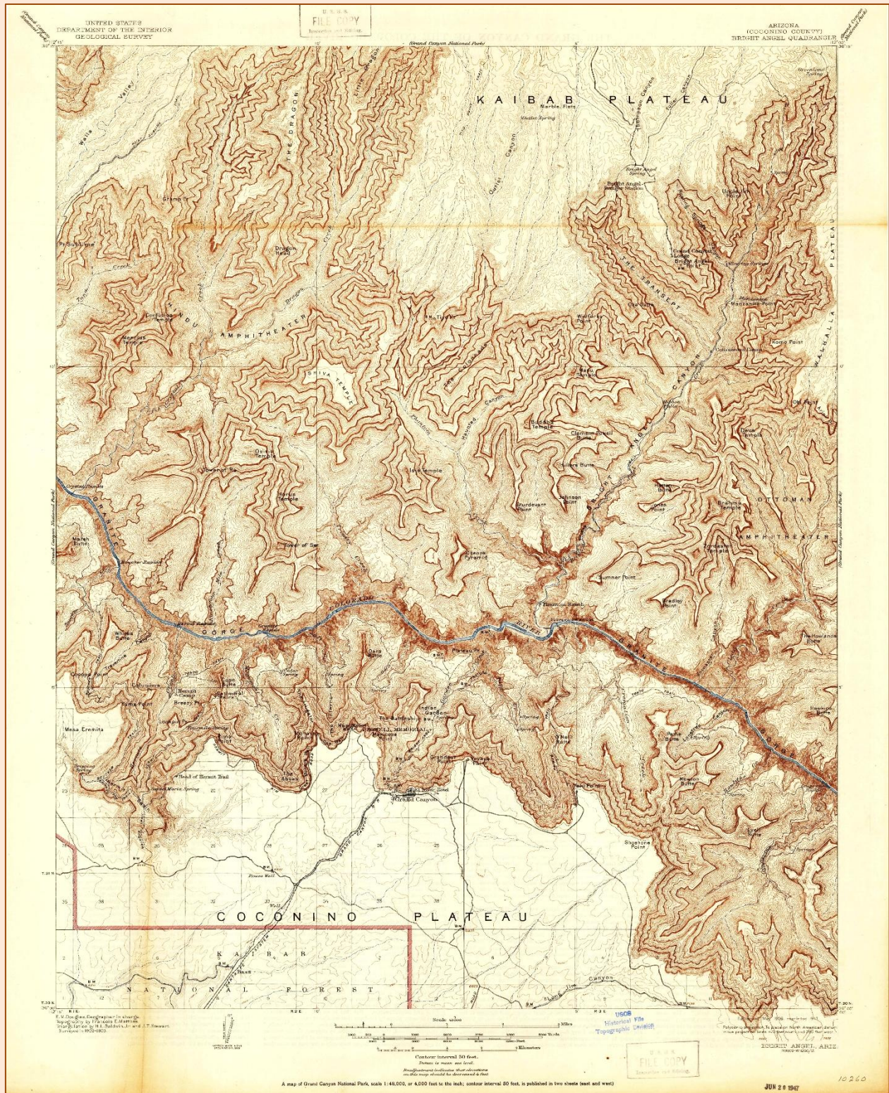
Figure 44. Bright Angel, Ariz., Quadrangle. Scale 1:48,000, contour interval 50 feet. (“E. M. Douglas, Geographer in charge. Topography by Francois E. Matthes. Triangulation by H. L. Baldwin, Jr. and J. T. Stewart. Surveyed in 1902–1903.”)
