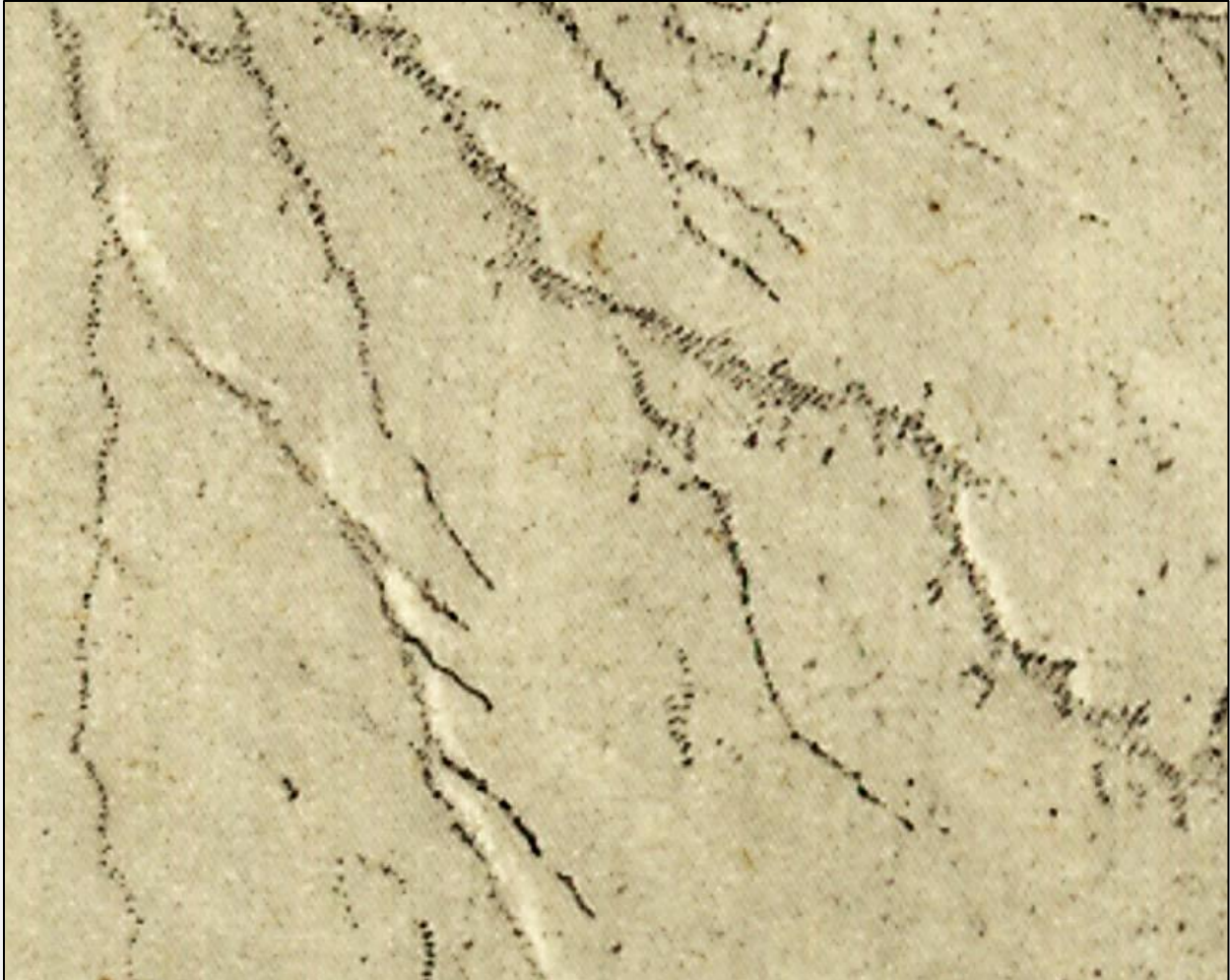
FIGURE 24. Very close detail showing parallel ruling as the result of using the very-fine-ruled glass screen, here showing the delicate headwater tendrils of shallowly excavated stream courses. This detail is from the headwaters of the Cataract Creek basin. Here one may see how the very fine ruling made light work of the depiction of comparatively shallow streamways scored on the plaster model, where hachuring would have been more time-consuming. [See also Appendix Figure A20. ]
