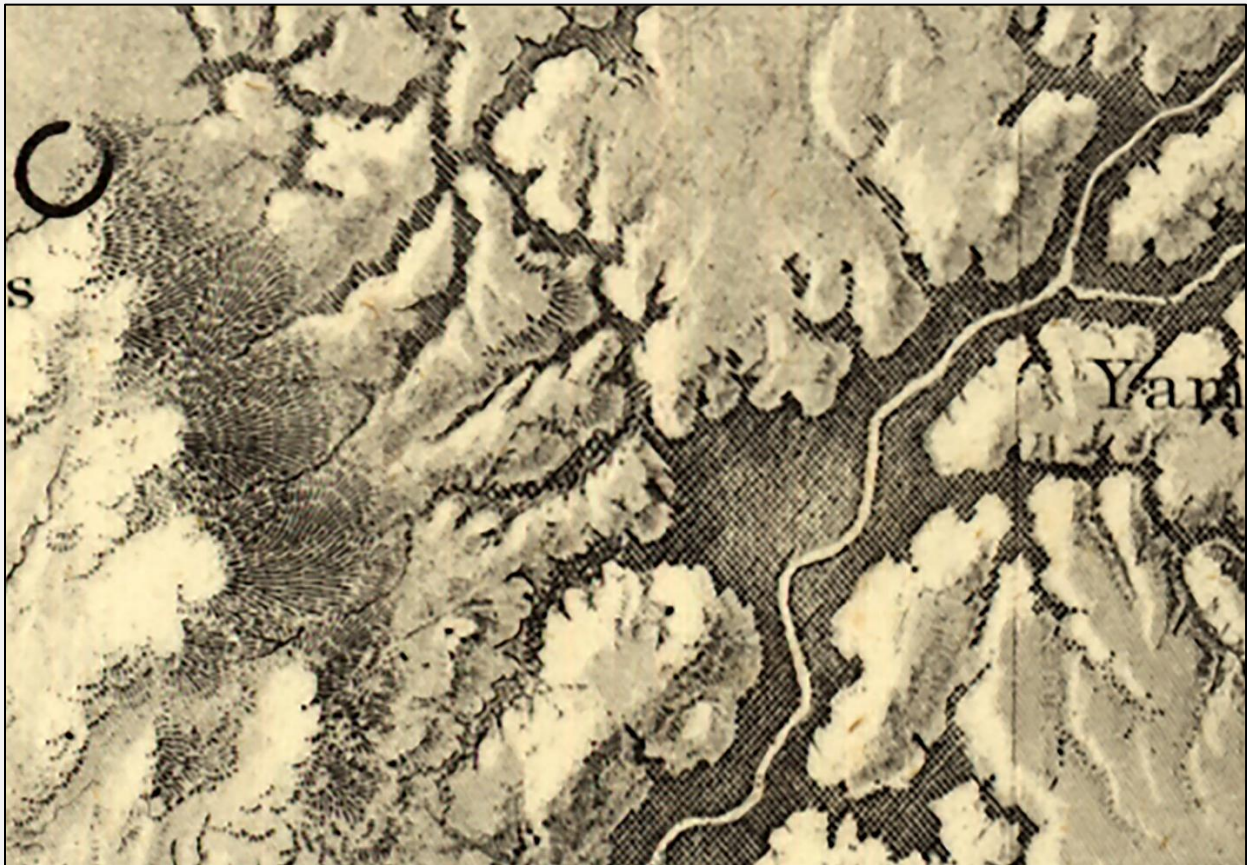
FIGURE 22. Hachuring and very fine criss-crossed ruling are seen side-by-side. The conventional sort of hachuring ( at left ), portraying the shaded side of a geographic feature, was used across Egloffstein's map (even though Ives' "Appendix D" had indicated that hachuring had been discontinued in the production of the Colorado Exploring Expedition's maps—a note intended to promote forthcoming advances in technique that Egloffstein was then improving). The criss-crossed ruling was reserved to show areas of deeper relief, including in the smallest of the convoluted tributaries. This fine detail is at the supposed confluence ( upper right ) of the Little Colorado River with the great Colorado. ♦
