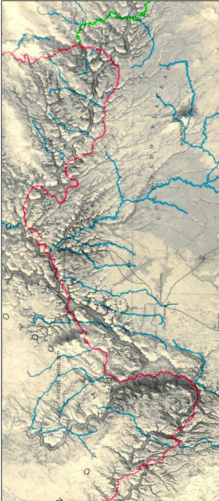
FIGURE 32. USGS Streamer river and tributary courses superposed on Egloffstein's map of the Grand Canyon. The Colorado River is here recolored red , and the Little Colorado River recolored green , in order to distinguish these streams from the blue -lined tributaries of the 1:1,000,000-scale Streamer map. The Egloffstein base map (in gray and pale yellow tints) reveals where his cartographical interpretations vary significantly from ground truth, particularly in the eastern Grand Canyon and in the vicinity of the unlabeled Parashant Wash basin on the west. Course deviations of the Colorado in the westernmost part of this detail, northwest of the Diamond Creek confluence (lowest arc on the west side here), are also pronounced though the two are in parallel. Red Butte is clearly misplaced westward and misleadingly enlarged on Egloffstein's map (see Appendix Figure A12 ). Note the dashed-line routes traveled by the Ives expedition ( lower part of map, left of center ), revealing that Egloffstein had had no vantages on the eastern half of this detail view. ♦
